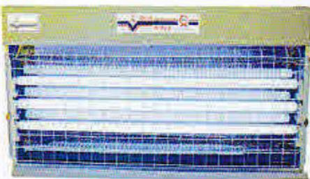
**INSECT KILLER** 6 lamps, each 40 watts, 120 cm in length, appliance height is 100 cms, operates on 220-250 volts AC 50-60 Hz/s, with a 200 watts high tension transformer and 1 pair of internal killing grids works both indoors and outdoors.
