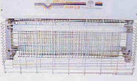
**STICKY BOARD** 2 lamps, each 20 watts, 60cm in length height 50 cms , 220-250volts AC 50-60 Hz/s, with sticky sheet for capturing flying insects, best used inside manufacturing lines, HACCP approved, body made of electrostatic treated metal, nice look, small size with high efficiency, works mostly indoors (More lamps means more power of attraction, & more coverage area)
